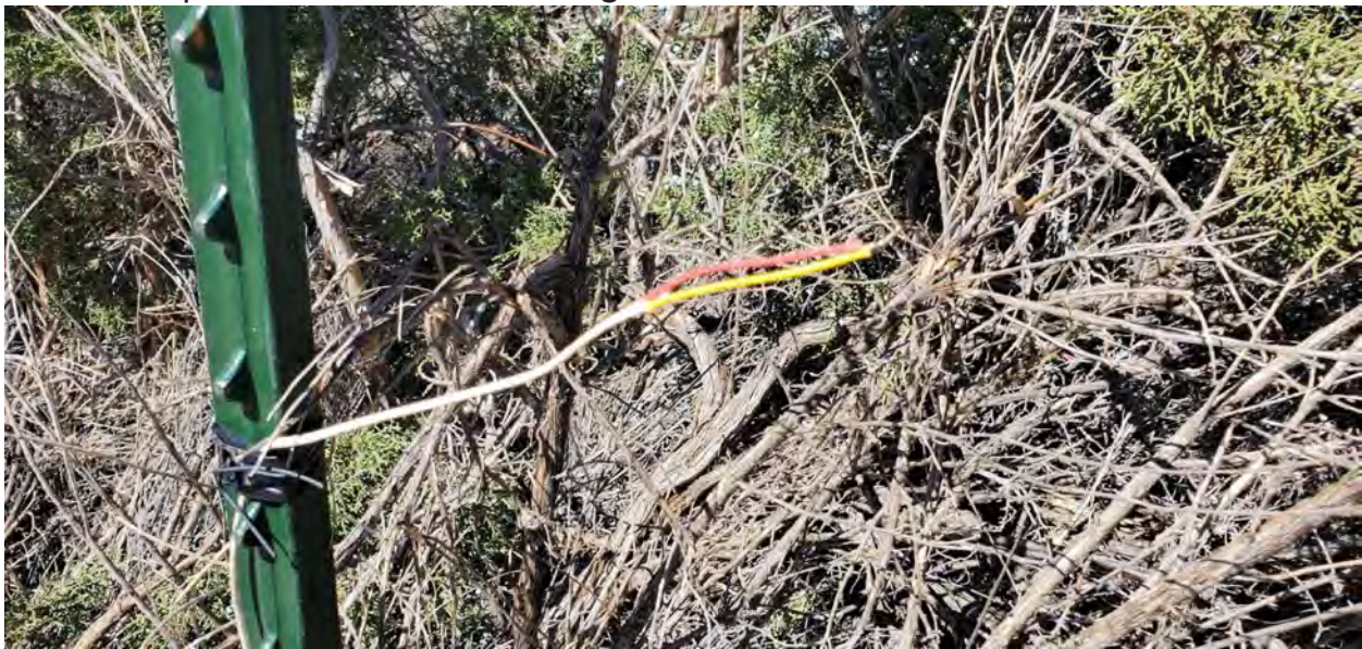
Photo showing steel post marker with Thermocouple installed at 4 feet above the ground surface
