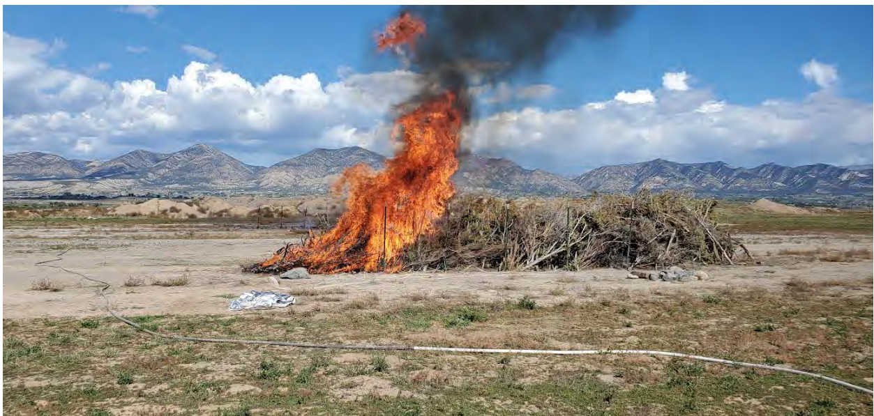
Time 1252: Fire has traveled from point ignition and well established at marker 1 and burning to marker 2. Flame lengths are approximately 18-20' and is burning intensely with little to no wind. The silver item in the foreground is a Wildland FireShelter being used to protect the data logger from radiant heat during the burn. Thermocouple wires run directly from the test locations to the data logger.
