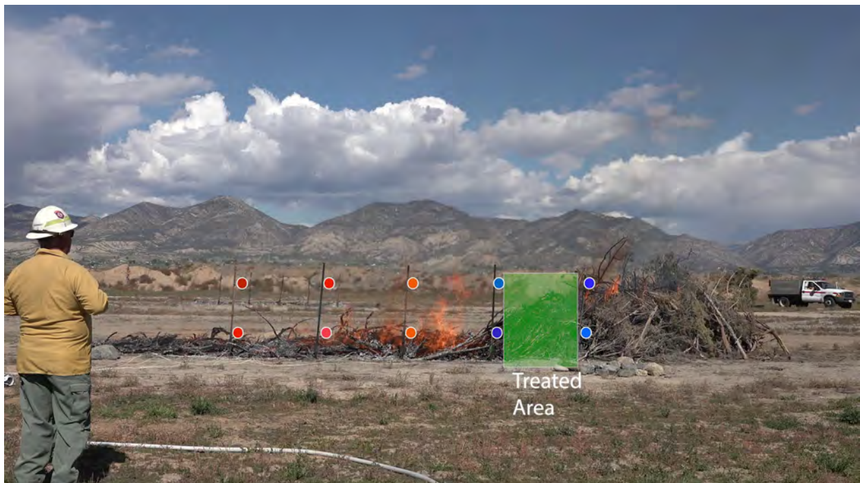
Time 1258: Photo shows effects of fire interaction with the suppressant. Fire is spreading past marker 5 into untreated fuels, but note the remaining large amount of unconsumed fuel between marker 4 and 5.
