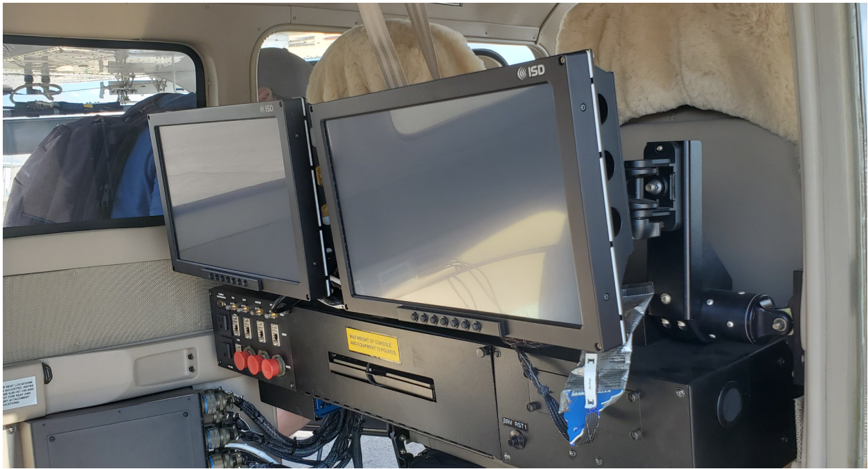
Figure 2: SAR Operator workstation on board the Cessna 206 aircraft. (CoE Photo)
