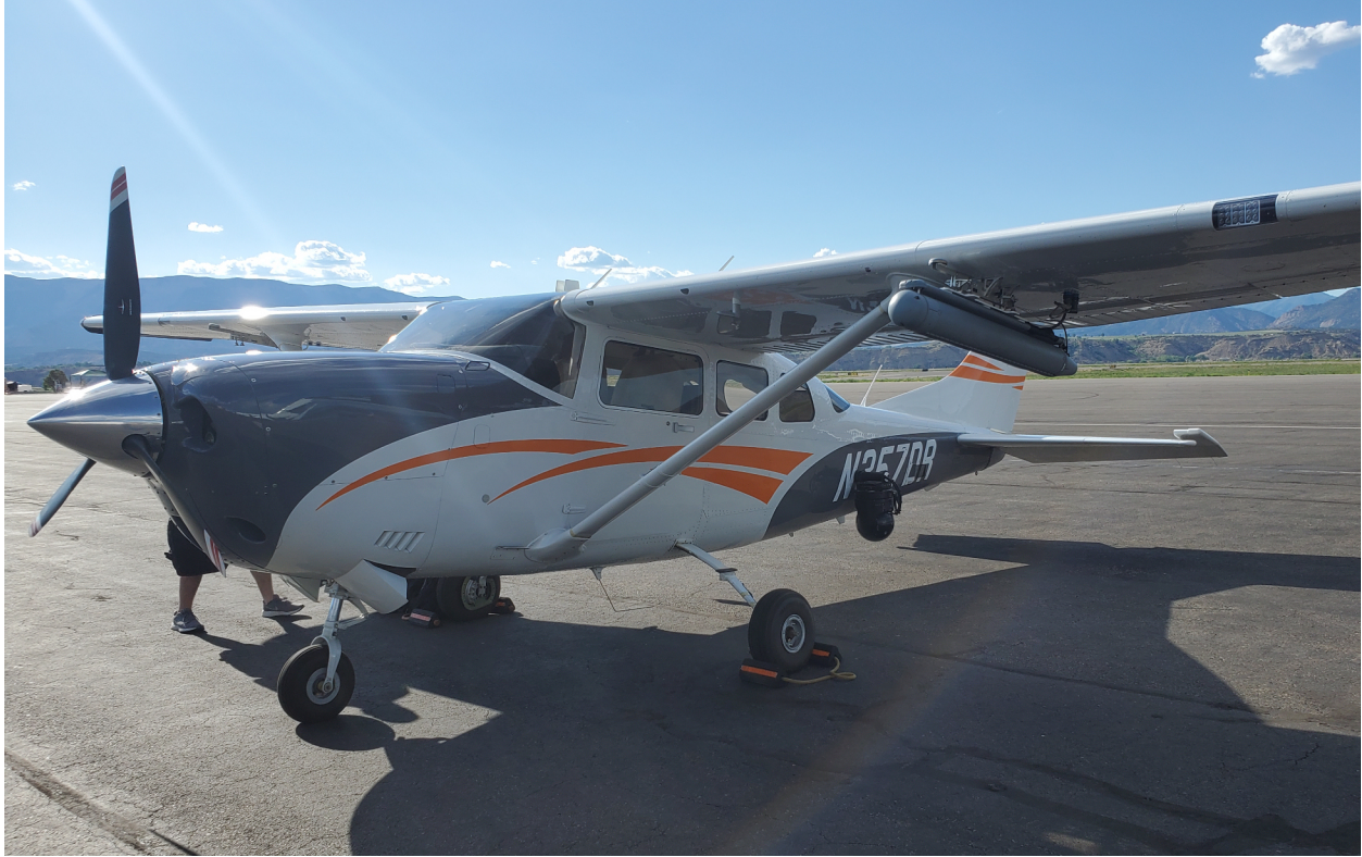
Figure 1: IMSAR's Cessna 206 below. NSP-7 Radar attached to the wing pylon (CoE Photo)
